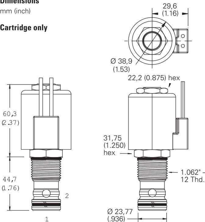
Torque cartridge in steel housing
