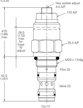
**Note:** Tightening torque of "F" adjuster locknut - 20 to 25 Nm
