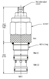
Turn CW to increase pressure setting and CCW to decrease pressure setting Torque lock nut to 20-25 Nm [15-18 ft lbs
