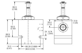
A Warning Maintain 5-8 Nm (4-6 ft lbs) maximum torque on valve tube nut.
