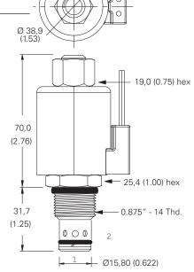
Torque cartridge in aluminum housing 47-54 Nm (35-40 ft lbs)
