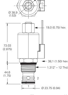
Torque cartridge in aluminum housing 108-122 Nm (80-90 ft lbs)
