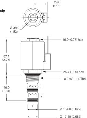
Torque cartridge in aluminum housing 47-54 Nm (35-40 ft lbs).
