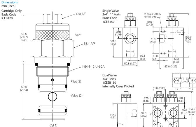
Note: For applications above 210 bar - please consult our technical department or use the steel body option .yi 1) Note: Tightening torque of "F" adjuster locknut - 20 to 25 Nm.
