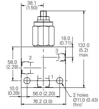
**Dual Valve** 1/2" Ports Basic Code 1CEEL95 Internally Cross Piloted)
