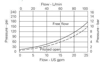
Note: This valve has been designed to eliminate instability from flexible boom applications or where the load induced pressure varies greatly. To get the best results, the settings should be adjusted for each application and then factory set for production quantities. Please contact our Technical Department for more information.
