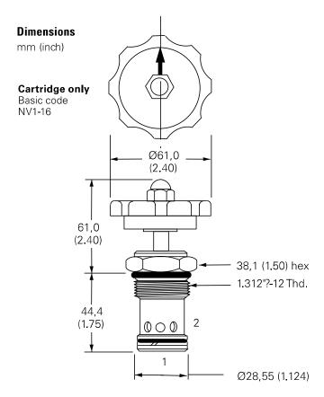
Torque cartridge in aluminum housing 108-122 Nm (80-90 ft lbs)
