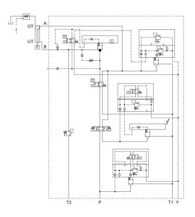
Example: PressPro up to size 63 (cartridge valves)
