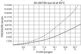
Performance with 12 VDC Coils and 10.3 bar/150 psi inline compensator (for other voltages consult factory)
