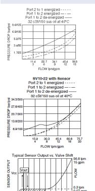
50 VALVE SHIFT % Hatched Area: Overlapping Stroke, Leakage Flow
